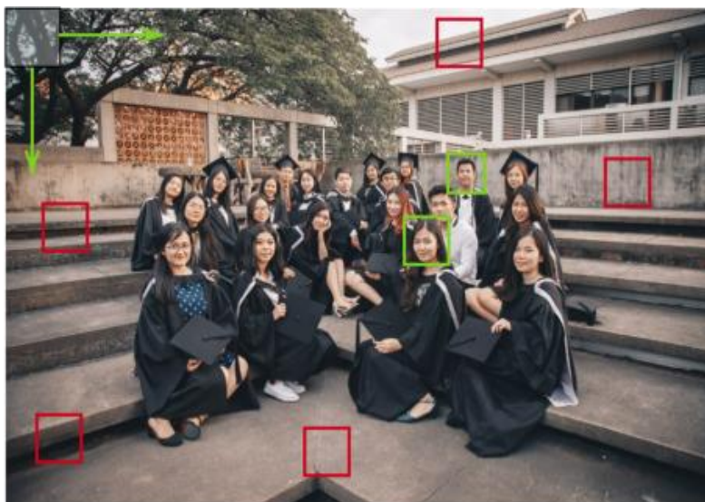
Figure 6 Sliding Windows Detection Process in the Viola-Jones Object Detection Framework
