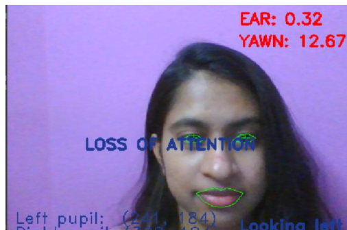
Figure 8, Eyeball tracking to detect loss of attention of the driver.
