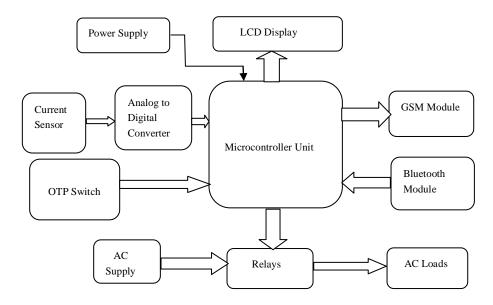
The system has a current sensor which will five load current value. Output of the CT is analog, so we have to connect a ADC in order to convert it in 8 bit Digital. This is done by using a ADC0808. Output of ADC can be fed to the microcontroller. Microcontroller will display the current value on a 16\*2 LCD. The controller will also compare it with the maximum allowable current value. If it is greater than that then the relay will get tripped automatically.
