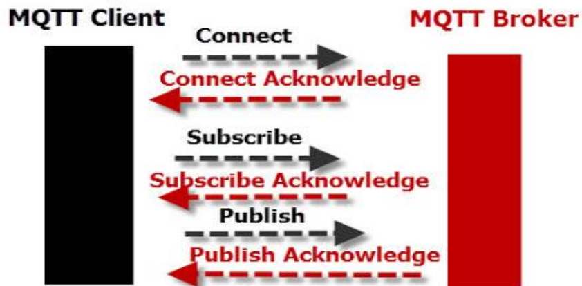
Fig. 2 - MQTT Client to Broker Protocol
